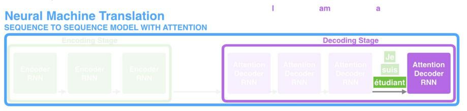
At time step 7, the attention mechanism enables the decoder to focus on the word "étudiant" ("student" in French) before it generates the English translation. This ability to amplify the signal from the relevant part of the input sequence makes attention models produce better results than models without attention.
